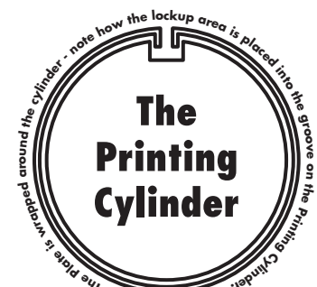
Below: The wrapping of the plate on the Printing Cylinder.
